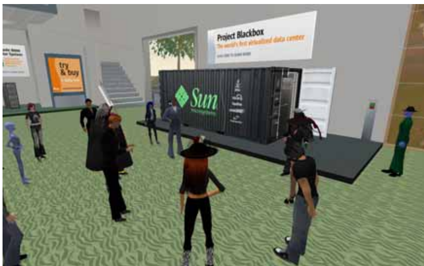
Sun Microsystem's Project Blackbox is a complete data center built inside a standard shipping container.
